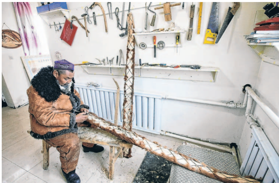
A craftsman makes traditional skis, with horse hair for going uphill, near the city of Altay, in China.
