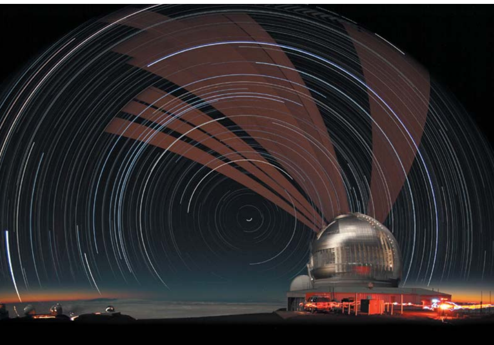
Gemini North fires a laser at the sky (shown in time-lapse) to correct for atmospheric distortions.
