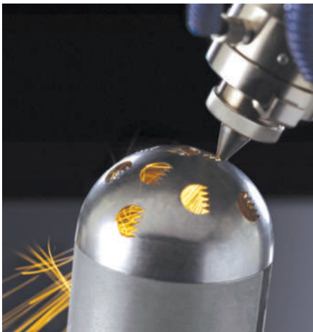
A solid-state laser cutting a series of fine patterns in a medical instrument.
