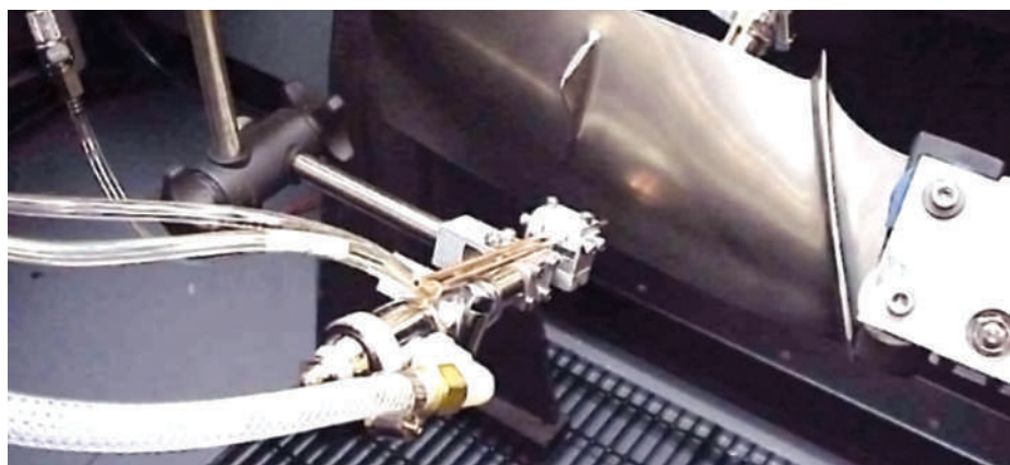
Figure 4 | LSP Technologies' RapidCoater system positioned for processing a turbine engine blade.
