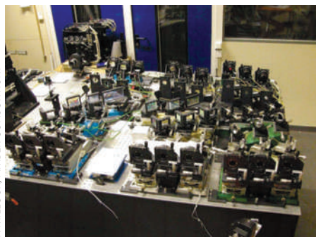
Figure 3 | Complex bulk optics: part of the VLT1 Amber instrument.
