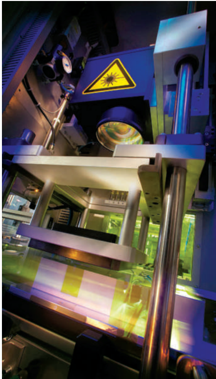
Figure 3 | Scanner-based welding system integrated into a conveyor line. The approach allows efficient mass production.
