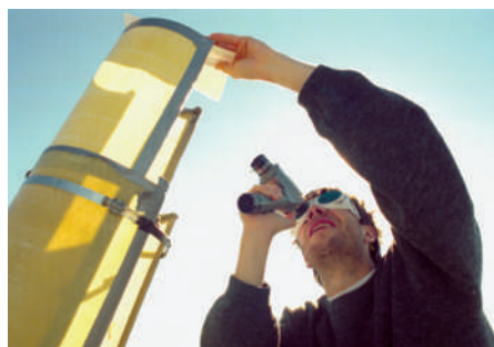
Jérôme Kasparian, leader of the Teramobile team, adjusts the beam path of the Teramobile laser.
