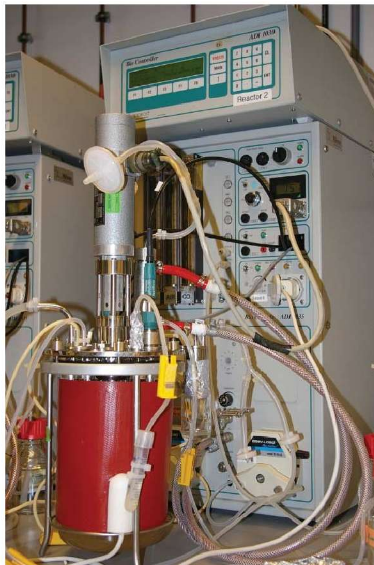
Relatively small bioreactors, such as these in the protein production core facility at EPFL, can produce large quantities of antibodies from traditional mammalian cell cultures. Image courtesy of F. Wurm.
